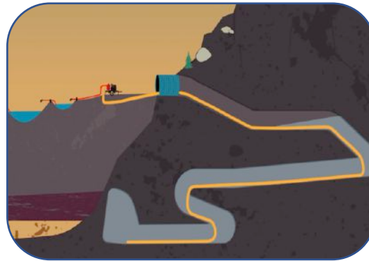
Dewater Existing Decline
