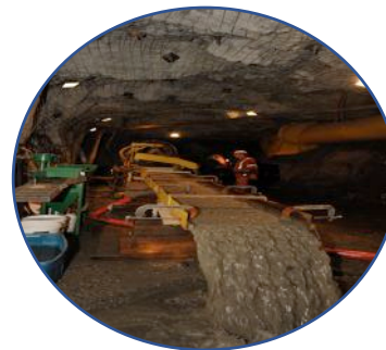
Crosscut Material Processed by Water Wash Plant Underground
