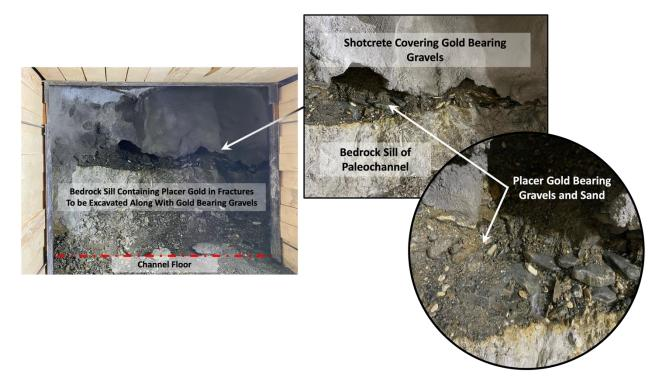
Fortis has temporarily paused this heading after successfully entering the paleochannel in order to advance the footwall access/haulage drift a further 20 meters downstream (to the left of above photos) having completed approximately 10 meters of that in the past week. Once the access drift is extended, Fortis will begin another crosscut and then advance into the heart of the channel on multiple headings to excavate the gold bearing gravels between crosscuts.
