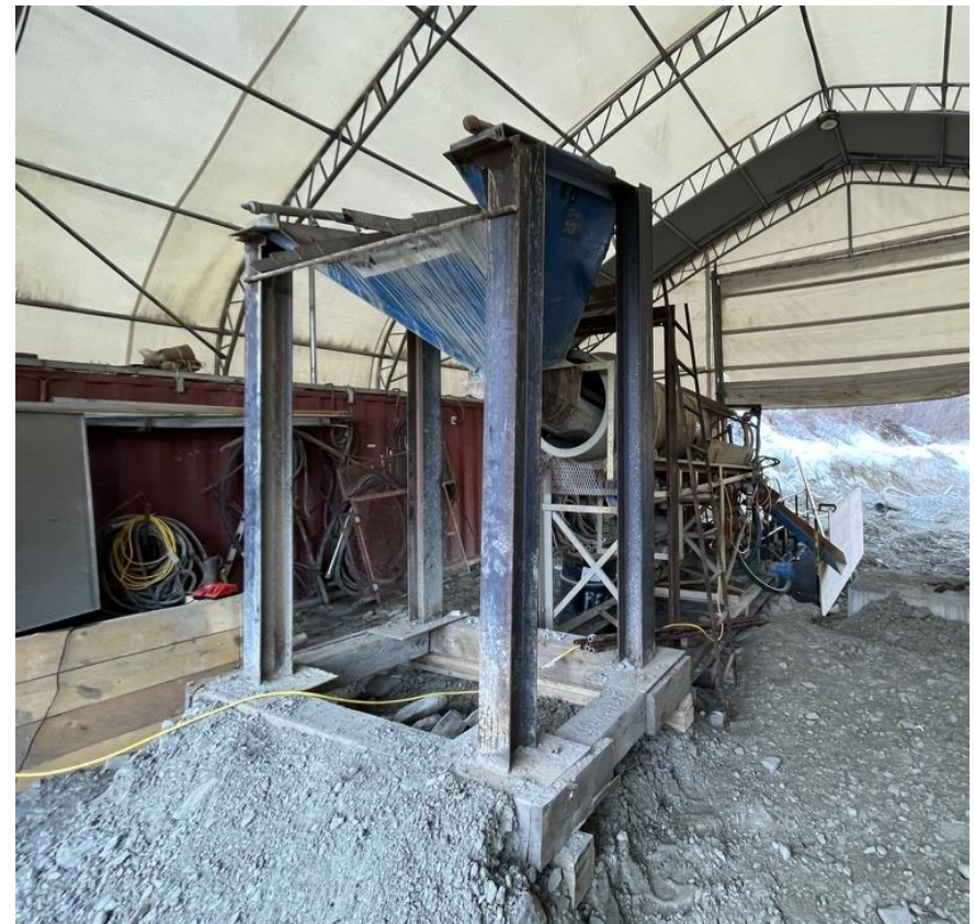
Frontend – Wash Plant Hopper
